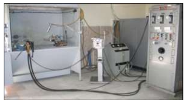
Figure 1: Plasma sprayed unit used in this investigation.
